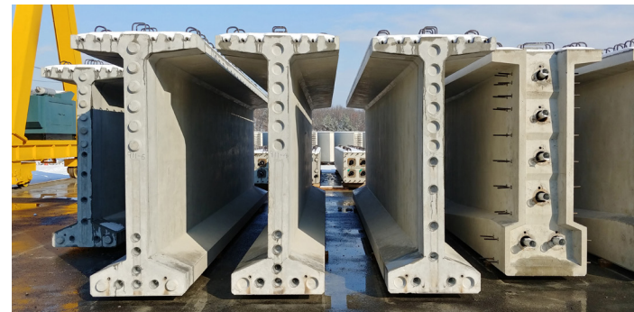
SegBeam _ Spliced PSC I Type Girder
