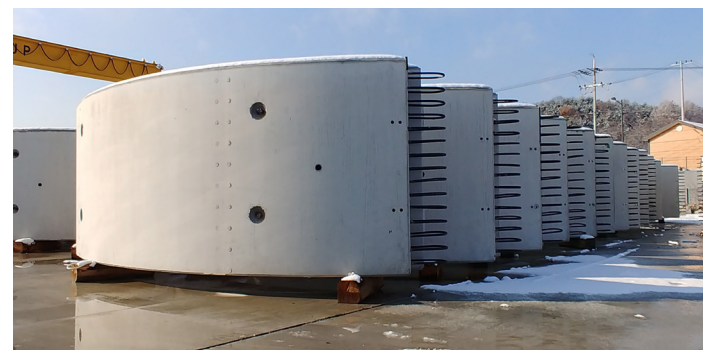
SegArch _ Precast arch for open-cut tunnel & bridge
